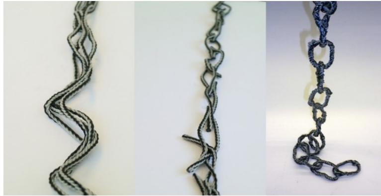
Fig. 10 Three production steps in the manufacture of a textile chain from left to right: braiding, cut braiding, ready-made braiding (manufacture on VF 1/(4-32)-140).
