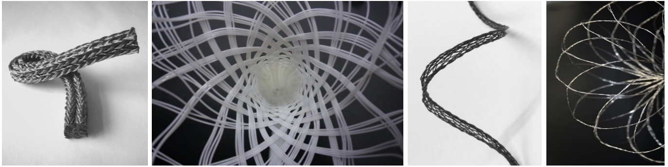
Fig. 2 Braiding options on the variation braiders – from left to right: packing braid, tubular braid, spiral braid, knotless net
