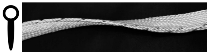
Fig. 13 Braided piping tape manufactured on a VF 1/(4-72)-140 (cross-section on the left side).
