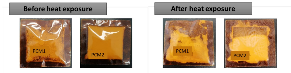
Fig. 5 Film PCM packages before and after heat exposure.
