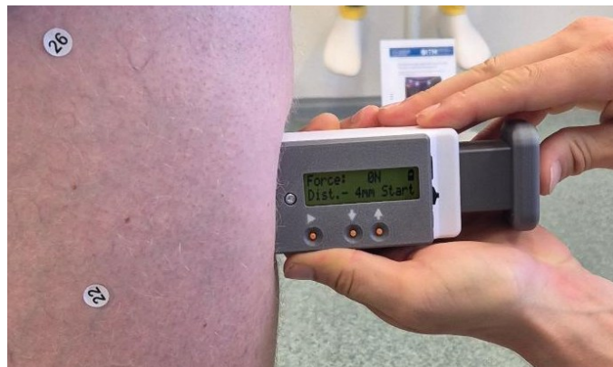
Fig. 4 Determination of soft tissue elasticity and penetration depth at a measurement point using the IdentoPRO device.
