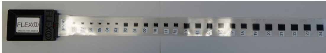
Fig. 6 Innovative Flexoo sensor with 24 wet cells, shown here as a development prototype
