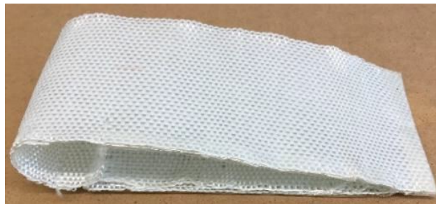
Figure 4: Basic weave with plain weave in all layers for the preliminary tests (left) and prototype made of glass fibers; manufactured on the semi-automatic laboratory loom (right).
