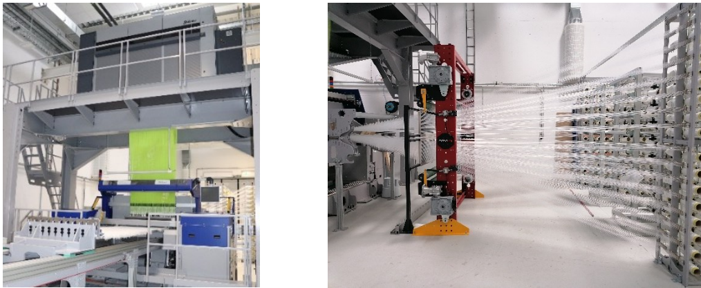
Figure 9: Double rapier weaving machine with single yarn control and linear take-off (left) and warp beam frame for two warp beams, as well as a creel with two special creels (Texmer) in the middle (right) at the textile technology center.
