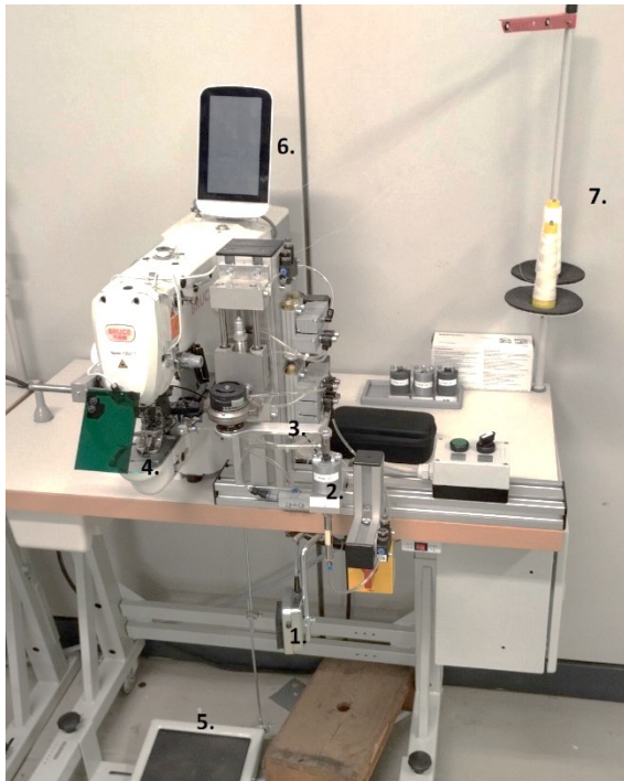
Fig. 6 Electronic high-speed button-sewing machine Bruce BRC-T1900G.
