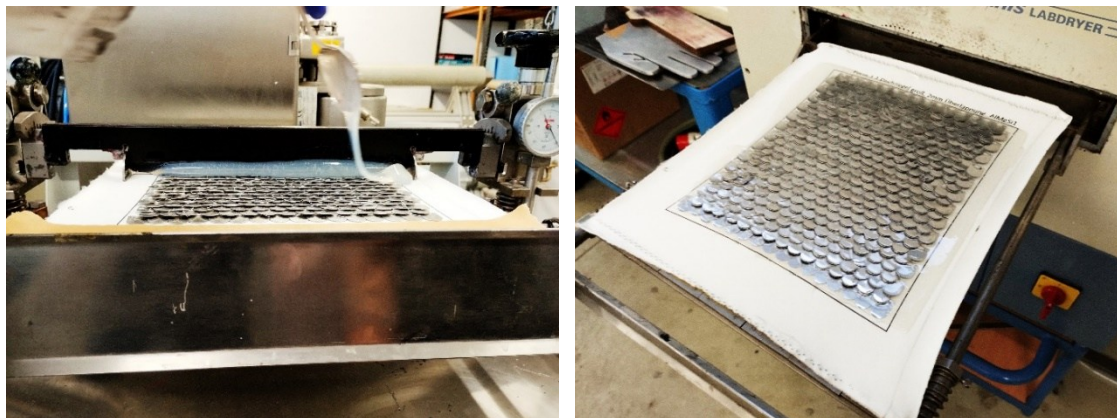
Fig. 8 Knife coating of the metal platelets.
