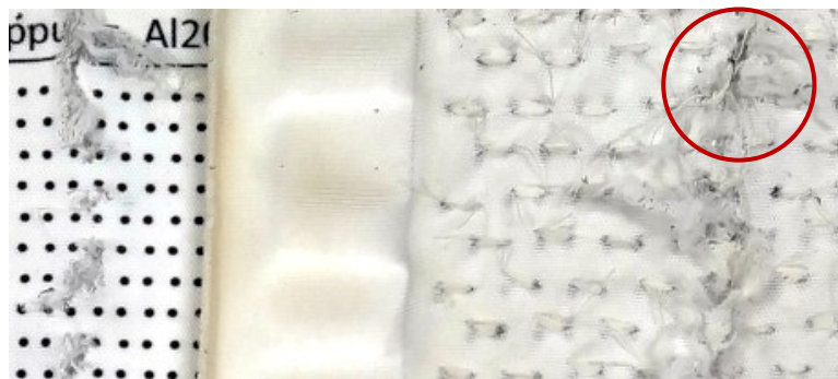
Fig. 12 Sharp corners of the platelets pierce and cut through the knitted fabric.
