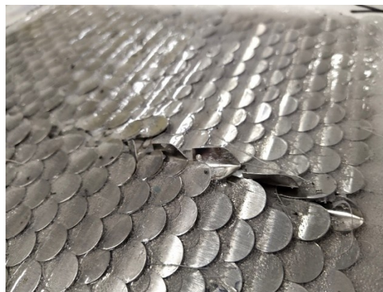
Fig. 13 Platelets are better fixed in place by a thin coating.
