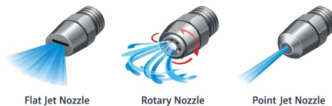
Fig. 3 Types of water jet nozzles (Image was generated using AI.).
